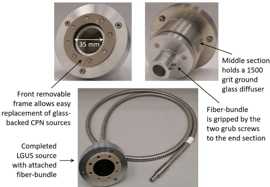
Fig. 1. Modular design of the LGUS source fabricated from aluminum. Clockwise: The CPN source element is securely held in a front plastic frame which is attached with screws to the middle section. The middle section holds a Thorlabs, Inc 1500 grit ground glass diffuser to both expand and homogenize the laser beam to a diameter of nearly 30 mm. The fiber-bundle is gripped by the two grub screws on the end section which in turn is secured to the middle section with screws.
