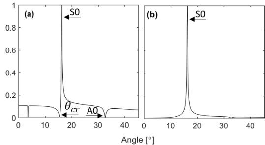
Fig. 4. (a) Integral of the normal strain component over the spacer thickness,  $\int(\partial u_z/\partial z).dz$ . (b) Integral of the transverse strain component over the spacer thickness,  $\int(\partial u_x/\partial z).dz$ . The profiles have been normalized to the maximum value.
