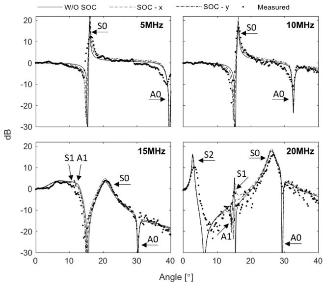
Fig. 2. Profiles of the measured and modeled directional response at four frequencies: 5 MHz, 10 MHz, 15 MHz and 20 MHz. Profiles of the measured data (points), modeled directivity excluding (solid) and including the SOCs have been plotted (polarized in  $x$  - dashed, polarized in  $y$  - dash-dotted). Features in the directional response correspond to the fundamental and higher-order symmetric (S) and anti-symmetric (A) Lamb modes.
