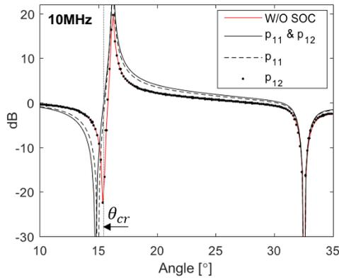
Fig. 5. Profiles at 10 MHz when including and excluding different SOCs. The model with the SOCs excluded (solid-red), the model with both SOCs included (solid-black), the model with only the  $p_{11}$  coefficient included (dashed) and the model with only the  $p_{12}$  coefficient included.
