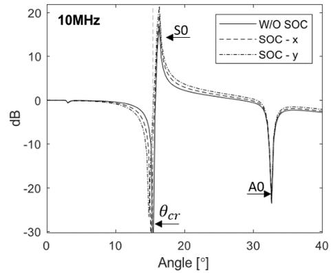
Fig. 3. Profiles of the modeled directional response at 10 MHz. Modeled directivity excluding (solid) and including the SOCs have been plotted (polarized in  $x$  - dashed, polarized in  $y$  - dash-dotted).
