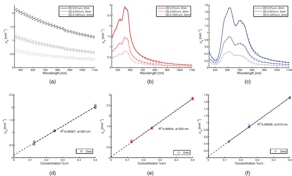
**Figure 4.** (a)–(c) Absorption spectra of PVCP slabs with embedded absorbers, at different concentrations; [S]—spectrophotometer acquired data. Dashed lines represent the standard deviation of the four measurements on the same sample. (d)–(f) Linearity of spectroscopic  $\mu_a$  with increasing concentration at the peak wavelength. (a) Black. (b) Red. (c) Blue. (d) Black. (e) Red. (f) Blue.
