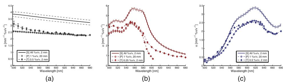
**Figure 6.** Comparison of extinction coefficient measured through: transmittance in spectrometer [S] (linear regression of results from samples at all concentrations) with cw-illumination, exponential fit of photoacoustic signal [P] and transmittance [T] with a high peak power OPO source. Measurement standard deviation is given. (a) Black. (b) Red. (c) Blue.
