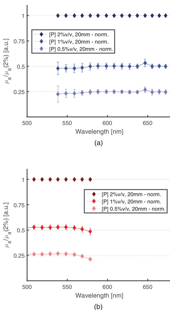
**Figure 8.** Spectra at different absorber concentrations (0.5, 1 and 2%v/v) normalised to the spectrum at 2 %v/v. 1/2 and 1/4 concentration ratios are broadly respected. Error bars account for inter-acquisition standard deviation and for the standard uncertainty in the exponential fitting procedure. (a) Blue absorber, (b) red absorber.
