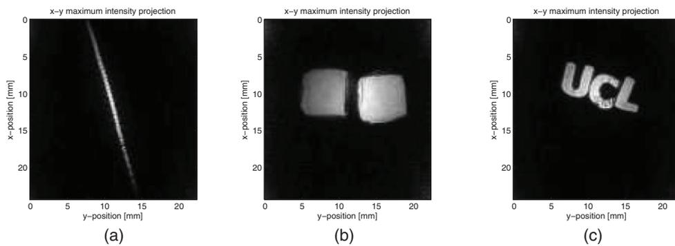
**Figure 10.**  $x$ - $y$  maximum intensity projections of the obtained PA images. In (b), the 2%v/v and 8%v/v black PVCP inserts are positioned left and right respectively. (a) Line phantom. (b) Embedded squares phantom. (c) 'UCL' phantom.
