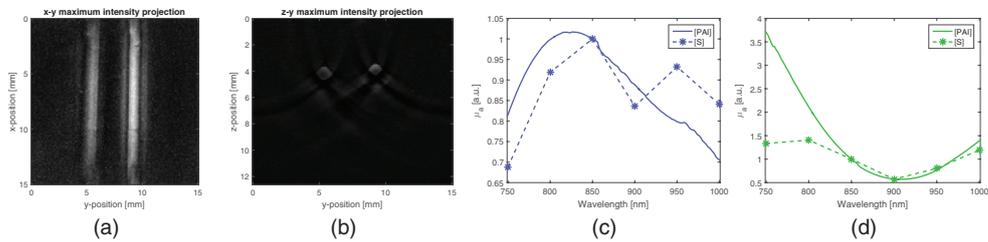
**Figure 11.** (a)  $x$ - $y$  MIP of a 3 mm slice for the channelled phantom, at 850 nm. Left:  $\text{CuCl}_2$ ; right:  $\text{NiCl}_2$ ; (b)  $y$ - $z$  MIP of the central 1 mm portion; (c)–(d) 850 nm normalised spectra for  $\text{CuCl}_2$  and  $\text{NiCl}_2$  respectively, comparing the spectrophotometer result ([S]) with the PAI intensity result ([PAI]).
