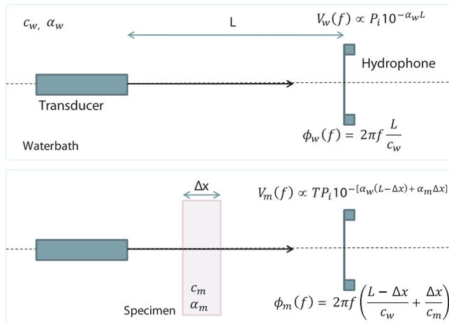
**Figure 1.** Through-transmission substitution setup used for sound speed and acoustic attenuation measurements.
