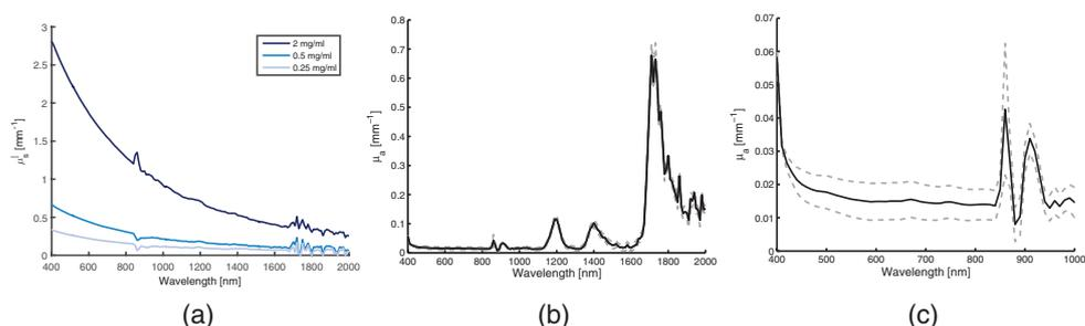
**Figure 3.** (a) Reduced scattering coefficient spectra of PVCP with varying concentrations of  $\text{TiO}_2$ . (b)–(c) Intrinsic absorption spectrum of soft PVCP. Variations at 850 nm are in fact artefacts due to the change of detectors within the spectrophotometer. The dashed lines correspond to the standard deviation between the estimated  $\mu_a$  for the four slabs.
