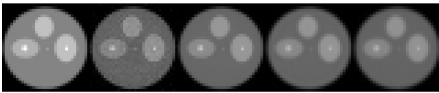
Fig. 7 Reconstructed z-plane at a depth of 0.25 cm reconstructed using noisy attenuated pressure, left to right: true phantom, SVD-based image, ideal-TR-based image, corrected-TR-based image, uncorrected-TR-based image.
