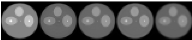
Fig. 4 Reconstructed z-slice at a depth of 0.25 cm of a 3-D phantom, left to right: true phantom, SVD-based image, ideal-TR-based image, corrected-TR-based image, uncorrected-TR-based image.
