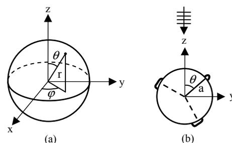
Figure 1. (a) General spherical coordinate system (b) Symmetrical coordinate system with incident wave in the negative Z-direction.
