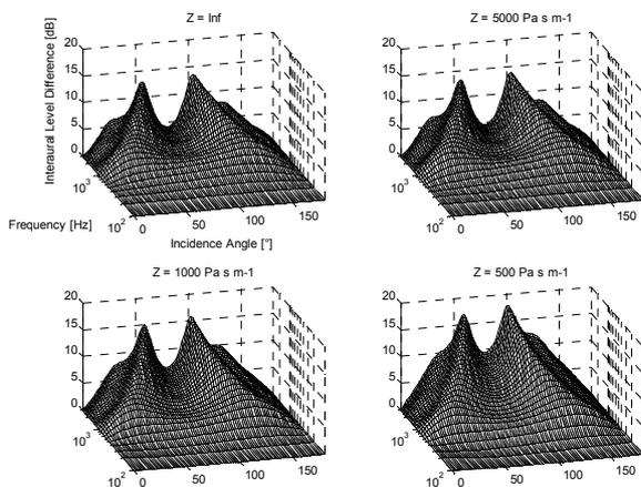
Figure 2. Increase in the interaural level difference with a decrease in resistive impedance.
