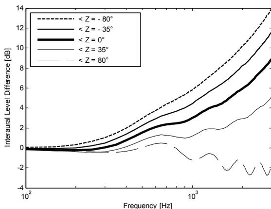
Figure 3. Change in interaural level difference with impedance phase angle for a constant impedance magnitude of 1000 Pa s m<sup>-1</sup> and a source angle of 90°.
